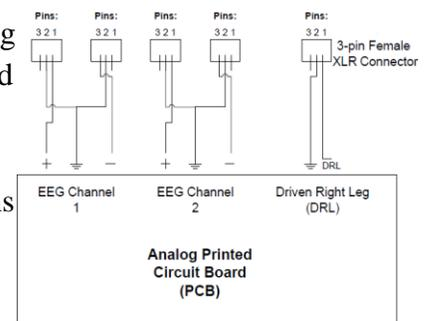
Figure 1: Analog Receiver Board and Connectors
